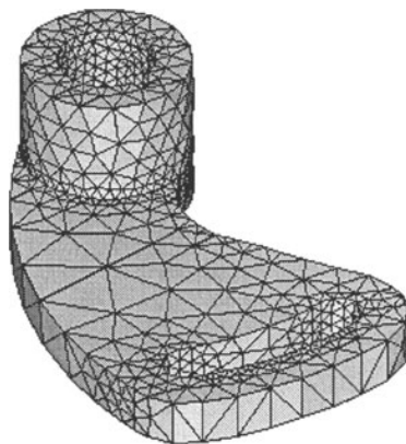
Example 1b: Command lever (pre-optimized) Number of triangles : 1944 Number of tetrahedra : 6013
