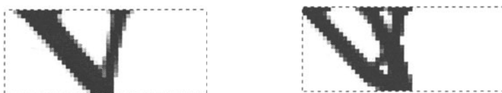
Figure 4. a) Min. of 'q-mean' of stress criteria and b) Min. of 'q-norm' of stress criteria.
