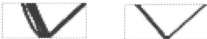
Figure 5. Minimum of maximum of local Ishai criteria a) T = 150 \text{ N/m}^2 , C = 450 \text{ N/m}^2 and b) T = 450 \text{ N/m}^2 , C = 150 \text{ N/m}^2 .
