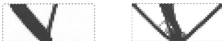
Figure 3. a) Min. compliance solution and b) Min. of the max. of the local von Mises stress.
