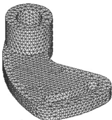
Example 1a : Command lever (constant density) Number of triangles : 3758 Number of tetrahedra : 10571
